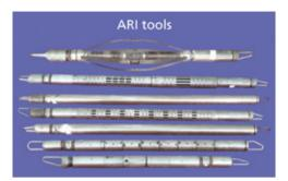
transmitting acoustic system, variable spacing, receiving acoustic system, receiving circuit and other subs. During logging, acoustic signals are sent from the sound source and enter into the formation, and then reflect when encounter small geological structures. The reflected signals are received by the receiving probe which amplifies the signals and sends them to the ground for record and storage. Then, special software is used for processing, analysis and identification.
