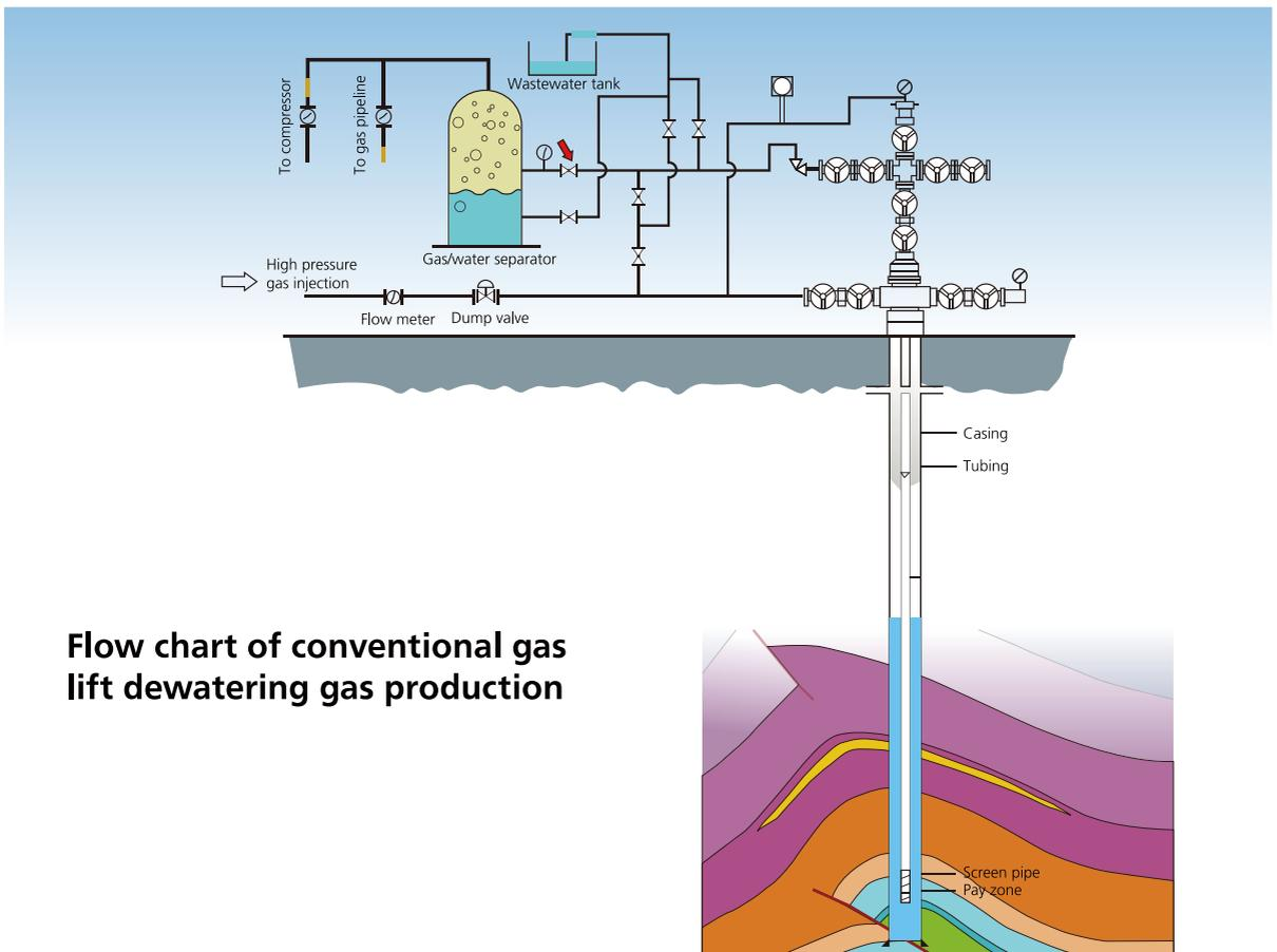
**Flow chart of conventional gas lift dewatering gas production**
