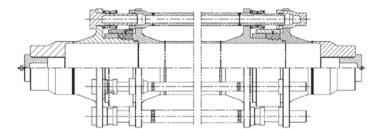
Assembly Diagram of the Flange Type Marine Riser for Pressure Test
