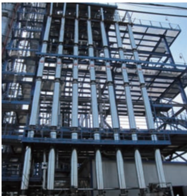
Tubular device of long term storage stability of modified oil from inferior heavy oil
