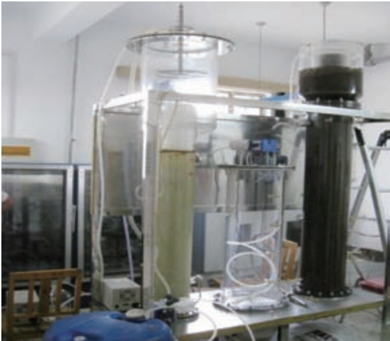
Test facility of loop flotation separation column
