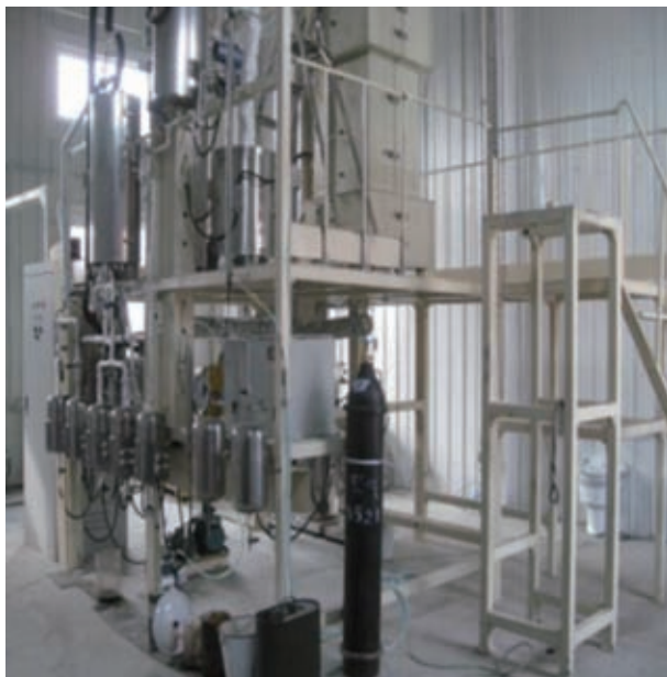
Pilot plant for viscosity reduction-coking
