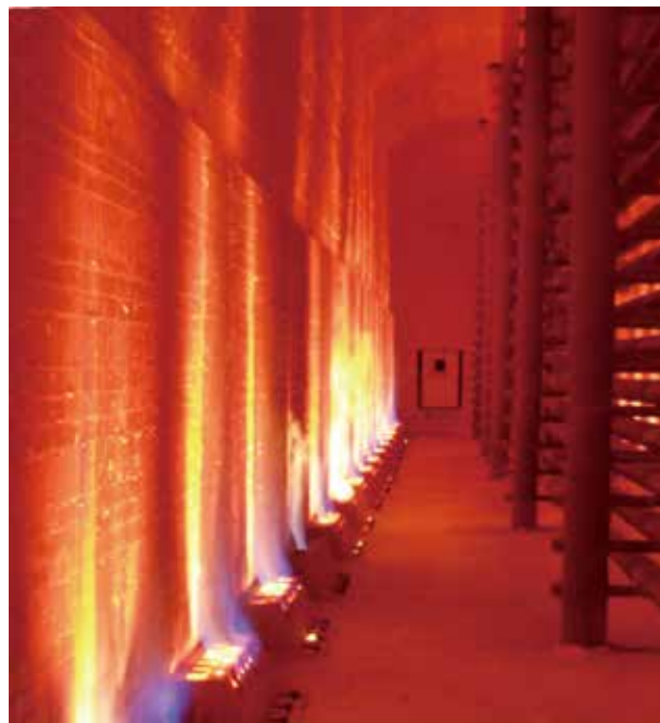
CNPC Liaohe Petrochemical Company's 100×10 4 t/a delayed coker with heating furnace modified by "wall-mounted furnace combustion technology"
