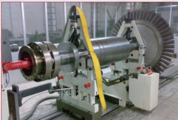
20t Rotor Dynamic Balance Test Machine
