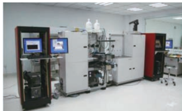
Combined HTHP Rock Electricity and Capillary Pressure Measuring System (RCS-763Z)
