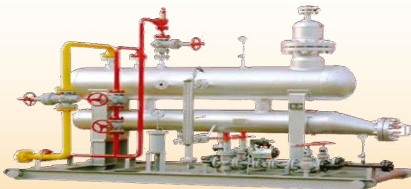
Gas-liquid separation skid
