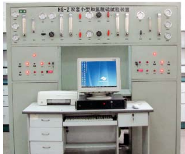
Hydrogen desulfurization experiment device
