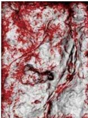
Coherence + fracture density Integrated fracture reservoir prediction result
