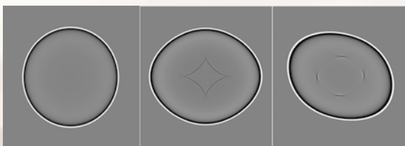
Seismic wave front comparison in isotropy (left), VTI (middle) and TTI (right) media
