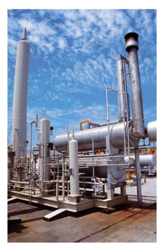
**Multi-well Heating Furnace** can heat multi-well at the same time and automatically adjust the water bath temperature. The thermal efficiency is more than 85%.
