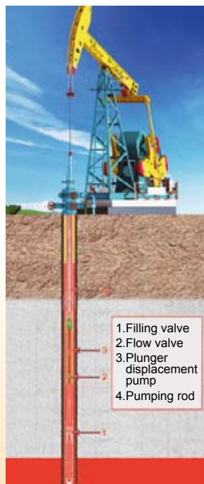
Sketch Map of Oil Production System for Pumping Unit—Plunger Displacement Pump
