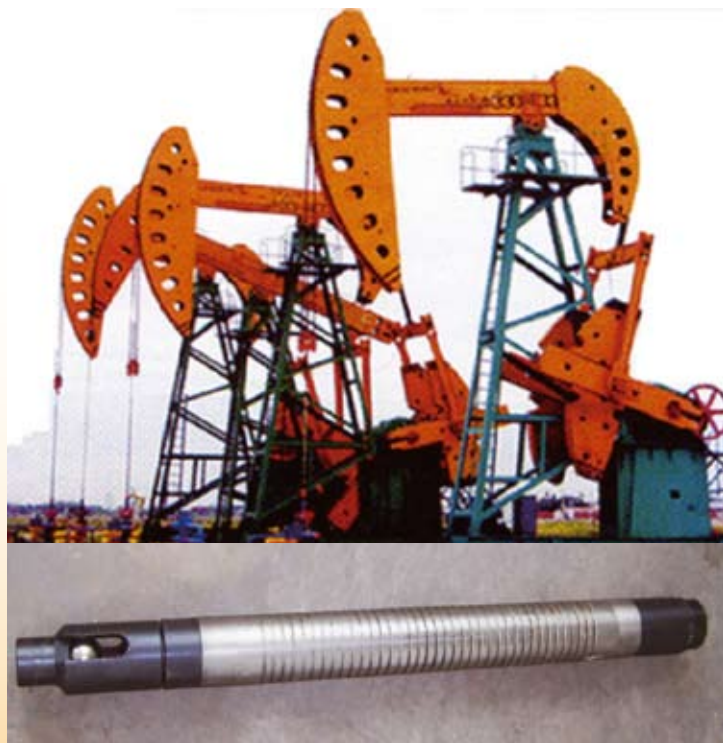
Pump plunger with low friction drag
