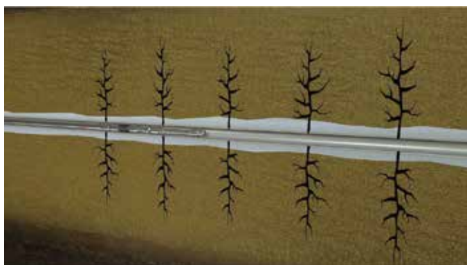
Schematic of hydrojet fracturing technology process in oil field
