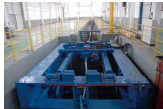
Physical picture of downhole tool experiment equipment for horizontal wells
