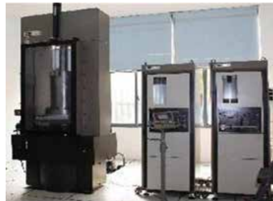
Physicals picture of MTS-815 three-axis rock mechanics testing system
