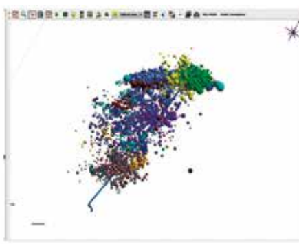
Top view of microseismic event positioning result of well N
