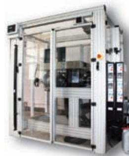
Pressure 70MPa, 380mL PVT barrel experiment device
