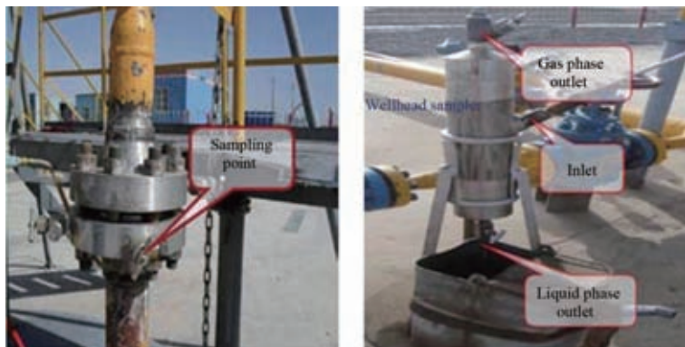
Fluid sampling unit diagram of Yaha condensate gas reservoir
