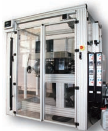
High-sulfur PVT instrument
