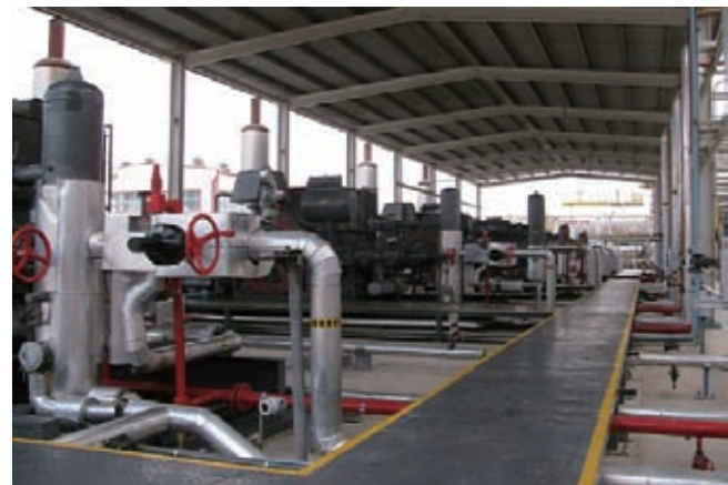
Medium pressure unit for gas injection in Yaha gas field
