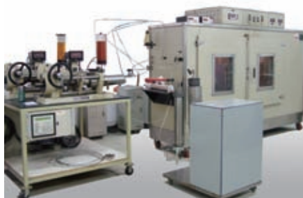
Long core gas injection displacement experiment equipment
