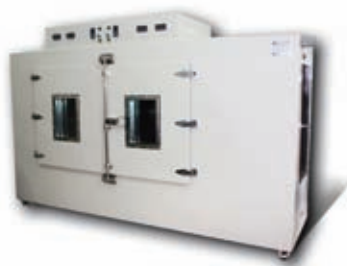
Pressure 70MPa, 380mL PVT barrel experiment device
