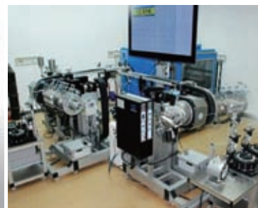
Miscible gas drive evaluation experiment equipment
