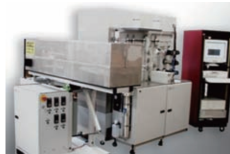
HTHP multiphase fluid percolation experiment Devices
