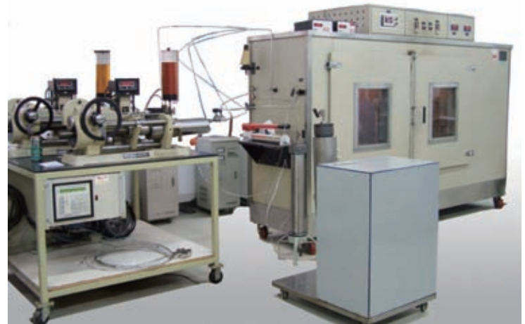
Long core gas injection displacement equipment
