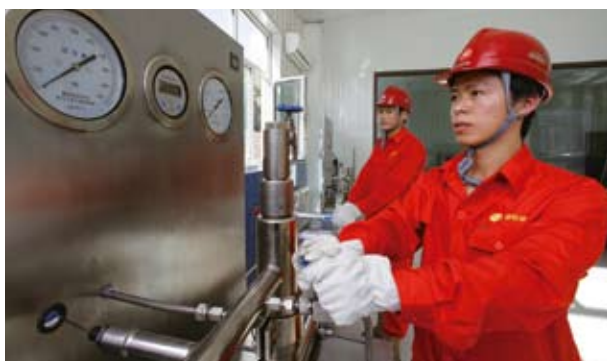
Commissioning table of gas-lift valve
