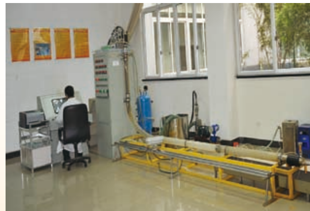
Horizontal well visualization simulation test unit
