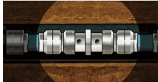
Differential pressure sliding sleeve opening
