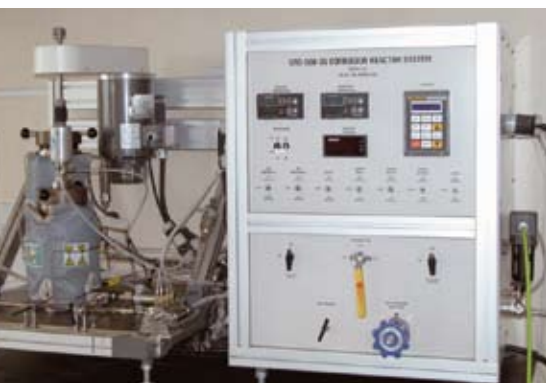
Rotating Disc Acid-rock Reaction Experiment Device
