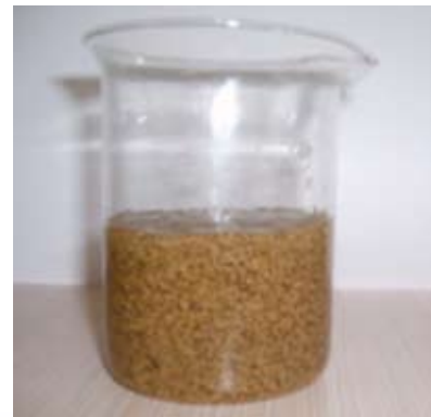
Sand Suspension Performance of Carboxymethyl Guar Gum Fracturing Fluid
