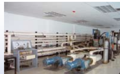
Multifunctional Pipeline Rheology Simulation Experiment Device
