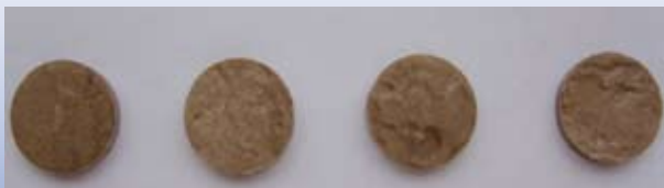
Etching Form of Core Surface After Reaction of Cross Linking Acid and Grainstone
