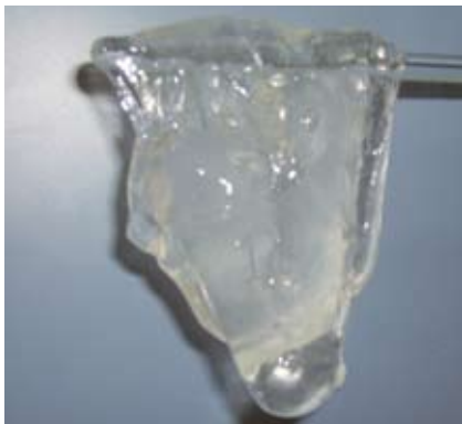
Hanging Performance of Carboxymethyl Guar Gum Fracturing Fluid
