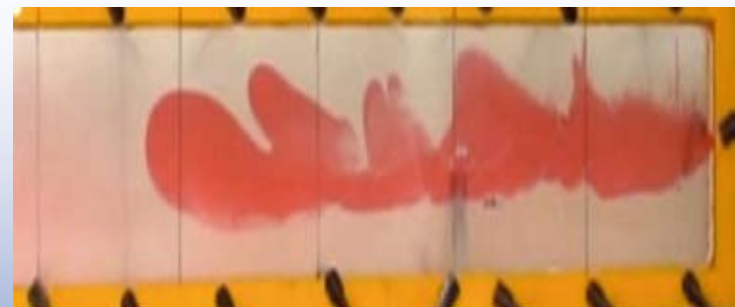
Large-scale Physical Model of Transparent Parallel Plates for Viscous Fingering Study
