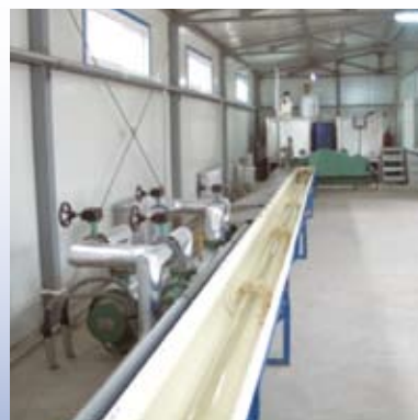
Large-scale Physical Model of Transparent Pipeline for Flow Regime Simulation Study for Horizontal Well
