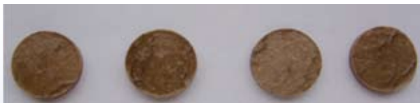
Etching Form of Core Surface After Reaction of Gel Acid and Grainstone
