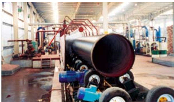
Anticorrosion operating line of steel pipe exterior
