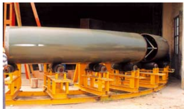
Anticorrosion operating line of elbow exterior
