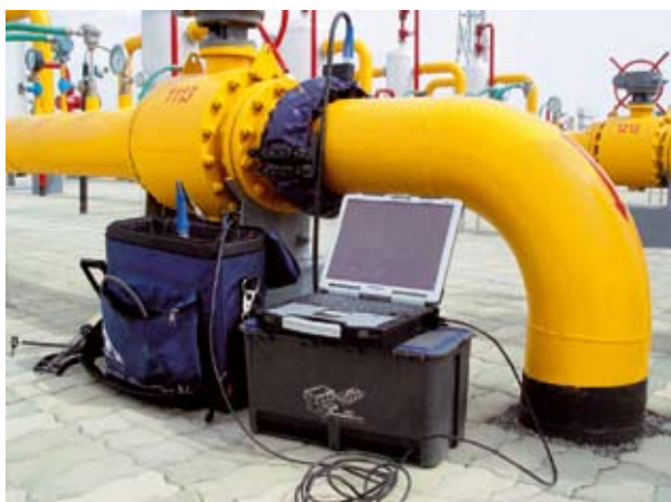
Utilizing ultrasonic guided wave testing equipment to test the defect of pipelines at the station
