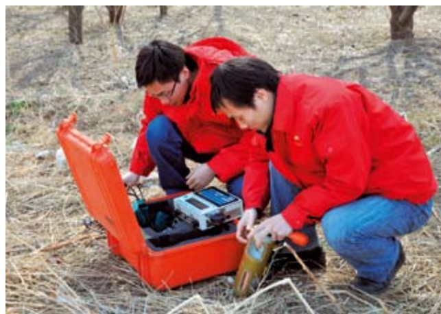
DCVG Survey along the pipeline
