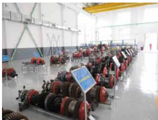
Figure 2-2 The intelligent pipeline detectors of different apertures
