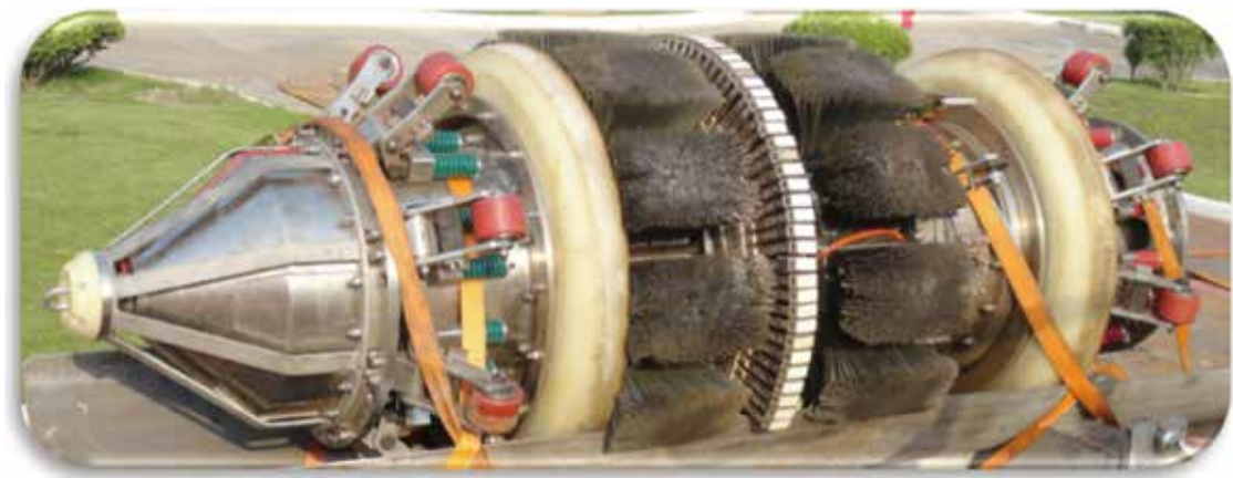
Figure 2-5 The \phi 1016 triaxial MFL corrosion detection with speed control system
