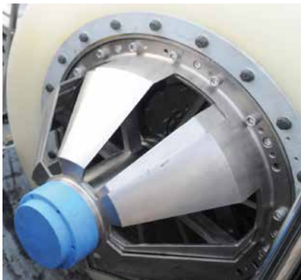
Figure 2-6 Opening of speed control system discharging device
