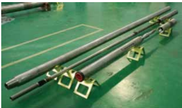
CGPWD downhole pressure measurement tool
