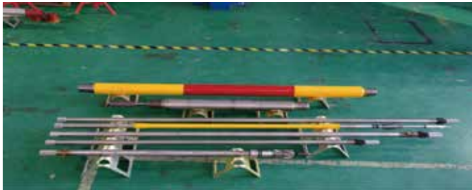
Generator, directional probe, EM signal transmitting unit, drill collar insulation transmitting antenna, azimuthal GR sub, etc
