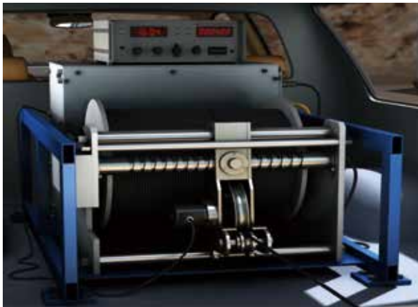
Surface IPC and cable winch
