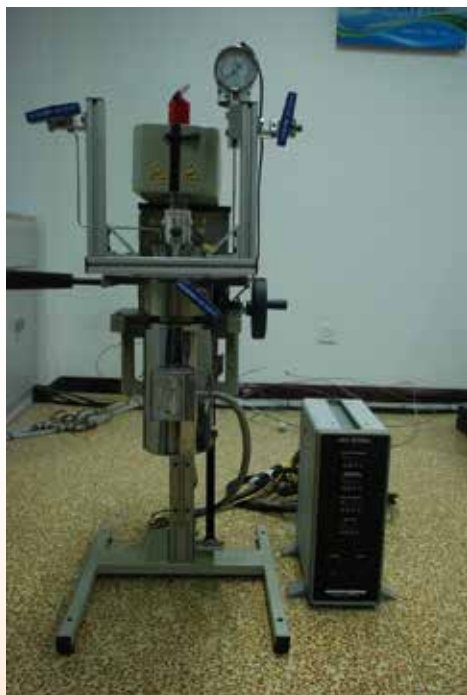
DR-7-002 microcomputer-controlled electrohydraulic servo pressure tester
