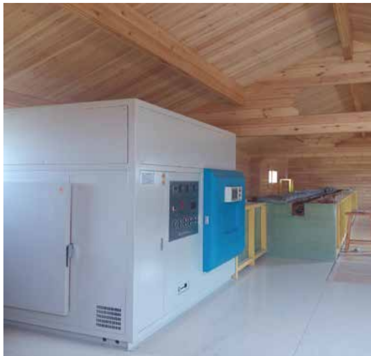
Large vibration table: used in vibration and impact test of cabinets and whole downhole tools and verification of vibration resistance and impact resistance of downhole tools, cases and cabinets after being well assembled and tested.
