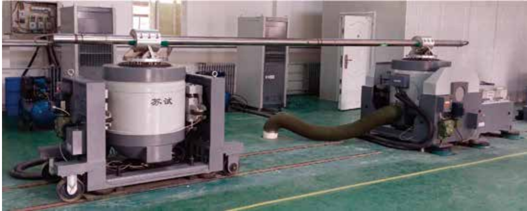
Large vibration table: used in vibration and impact test of cabinets and whole downhole tools and verification of vibration resistance and impact resistance of downhole tools, cases and cabinets after being well assembled and tested.
