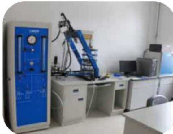
Dynamic triaxial shear equipment for earthwork
