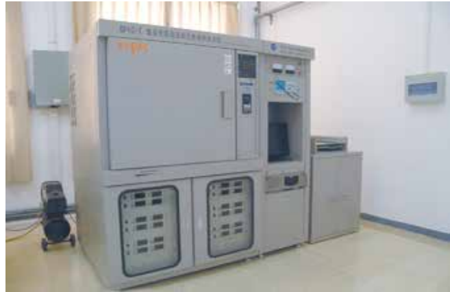
(SPIC-T) high temperature dynamic testing system for integrated circuits
