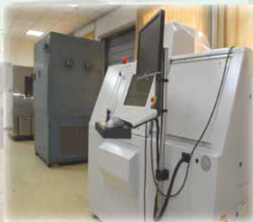
Micro-focus X-ray welding spot testing system (PCB analyser 160)
