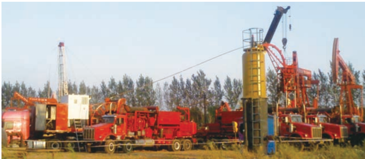
Hydraulic jet sand fracturing operations in well R72-24-38 in Liaohe oilfield
