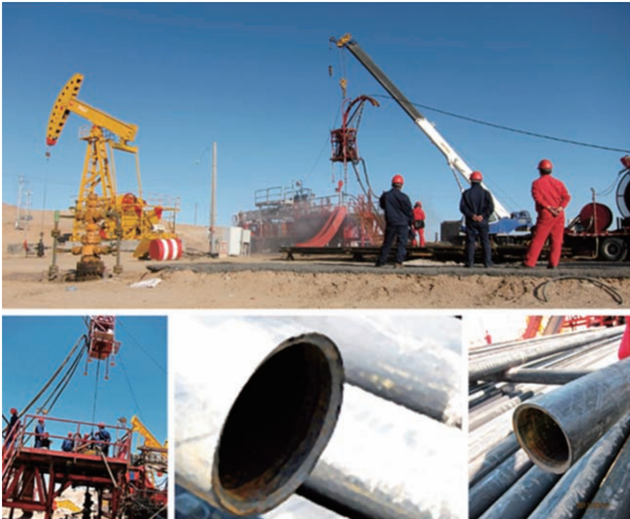
Hydraulic cutting of downhole tubing in Qinghai oilfield
