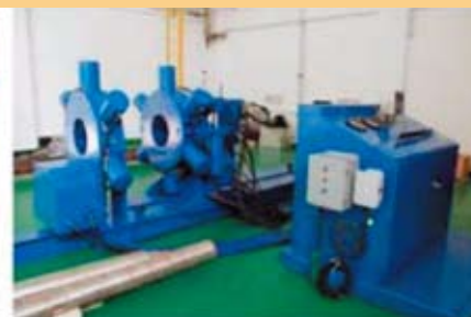
Removal and Mounting Machine for Downhole Instrument and Tools of MWD
