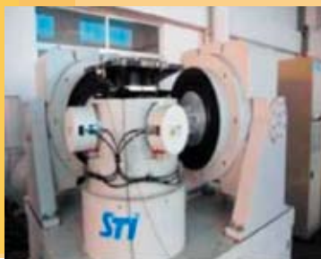
Test System of Electric Vibration for Triaxial Synchronous Vibration
