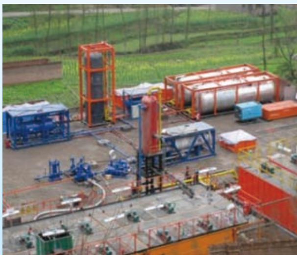
105MPa high sulfur-resistant two-phase flow and three-phase flow surface metering equipment
