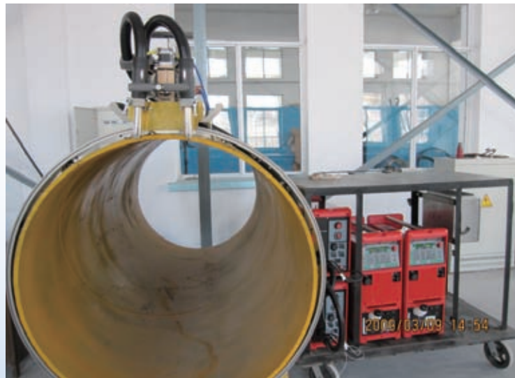
PAW3000 Double-torch all-position automatic pipeline external welding machine
