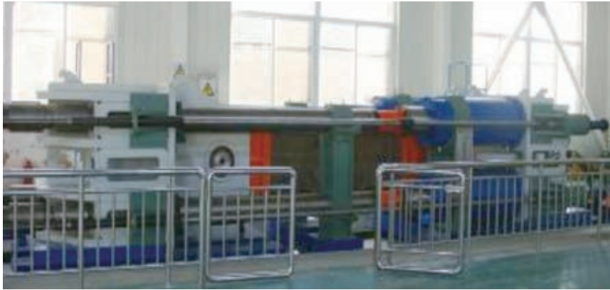
2000t Wide plate tensile test machine
