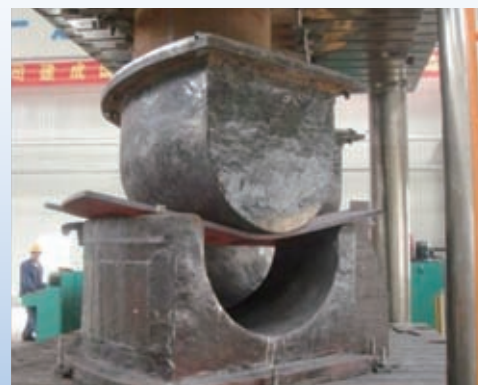
Pressing of hot-press elbow strap
