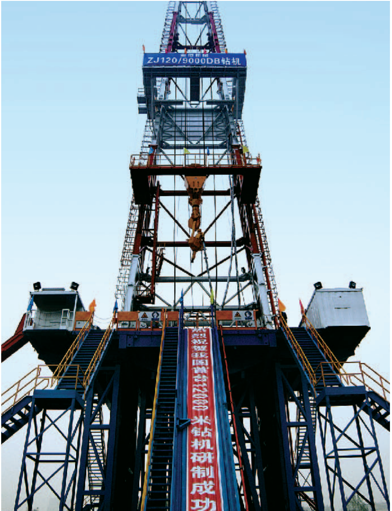
CNPC independently developed a drilling rig for ultra-deep wells, with a rated drilling depth up to 12,000 meters.
